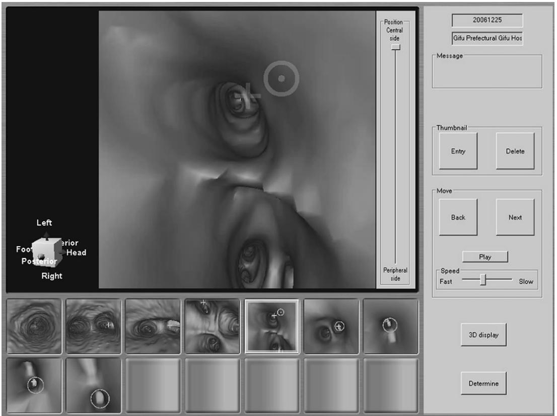
**Fig. 3.** VB image production, thumbnail registry. VB images of the path are automatically produced. While VB images are peripherally advanced, the bronchus for insertion is marked (cross) at each branching and registered as a thumbnail (lower area of the figure). The circle indicates the direction of the target.
